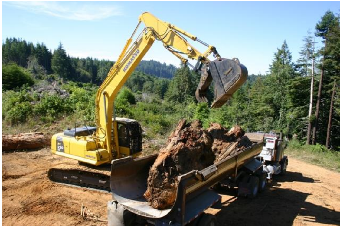
Figure 10. YTFP loading salvaged LWD into end-dump truck for transportation to the stockpile area, McGarvey Creek, Lower Klamath River, 2008.
