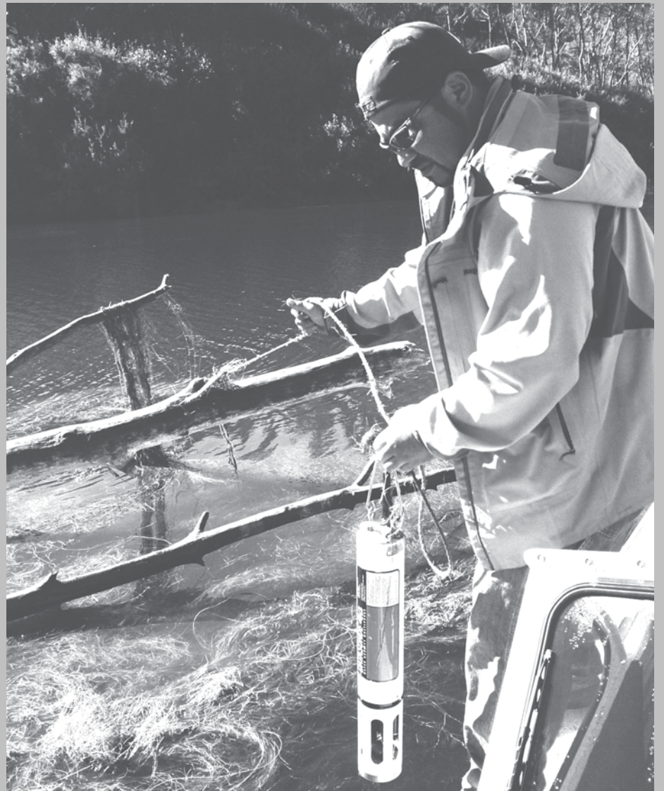
YTEP’s Micah Gibson deploys a data sonde in the Klamath Estuary.
