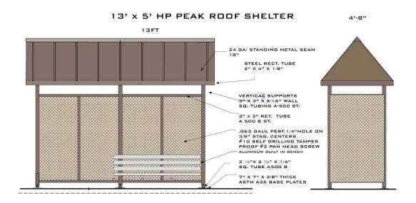
The basis of design for this report is governed by the provisions of ASCE 7-16 & the 2019 California Building Code. Through this report, it is shown that the proposed structure and anchorage to foundation elements establish a complete load path to resist the design loads prescribed by the governing codes and meet the requirements of the appropriate material specifications.
