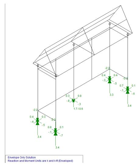
Per results above, the envelope reactions with overstrength factor. The worst case is Node16: Uplift Load = 2,300 lbs. Shear x = 100 lbs. Shear y = 800 lbs. Klamath Bus Stop **Project** Structural Calculations **Description** 11.01.2021
