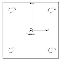
Anchor forces are calculated based on the assumption of a rigid anchor plate.
